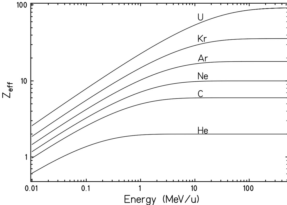
Fig. 4:  $Z_{\text{eff}}$  as function of particle energy. With increasing particle energy more electrons are stripped off and  $Z_{\text{eff}}$  approaches the atomic number  $Z$ .
