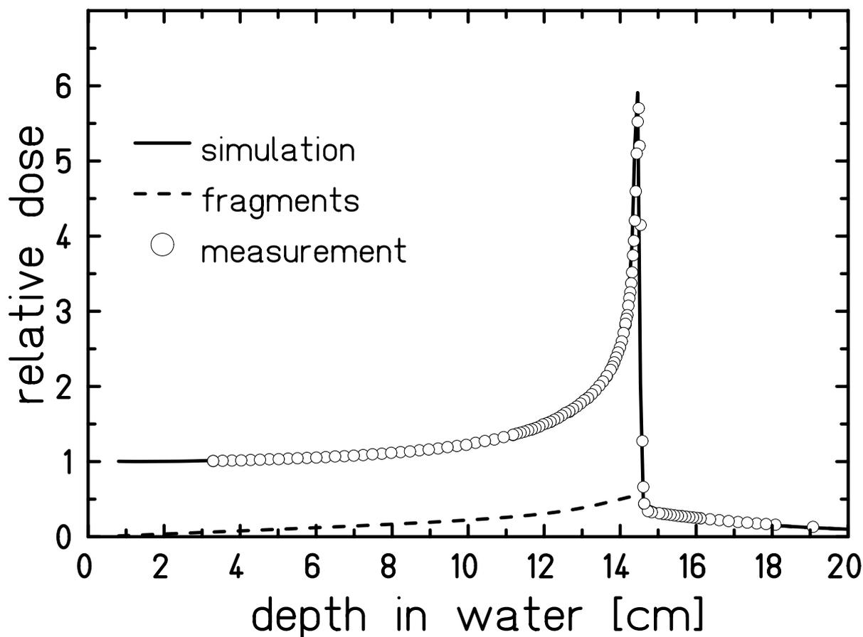
Fig. 7: Bragg curve of 270 MeV/u carbon ion. Measurements are compared with calculations including the contribution from nuclear fragments.
