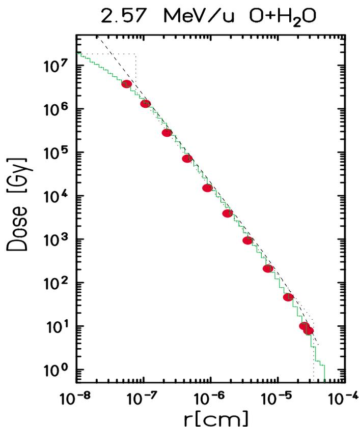
Fig. 9: Radial dose distribution inside a particle track according to different calculations are compared to measurements [Krämer 1994]
