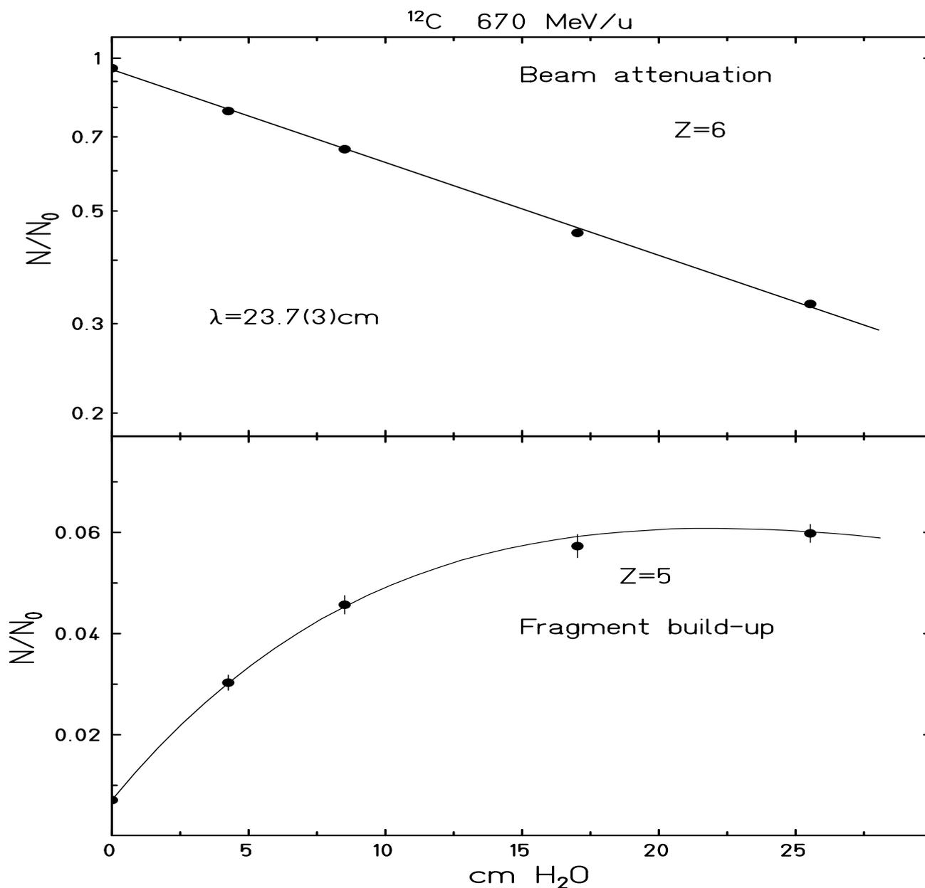
Fig. 6. Fragmentation of a 670 MeV/u carbon beam in water [Schall 1994]. Top: attenuation of the primary carbon beam as function of the penetration depth yielding a mean free path length  $\lambda = 23,7$  cm. Bottom: Build up of Boron ion fragments. Because of further fragmentation to lighter ions the intensity of Boron levels off for larger penetration depths. [Schall 1996]
