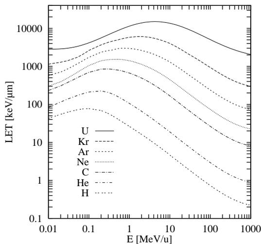
Fig. 3: Energy loss of different particles as function of the energy, calculated with ATIMA [Schwab 1991].
