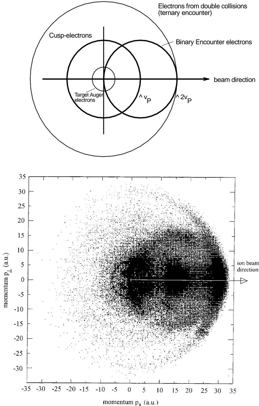
Fig. 10: Top: Velocity coordinates of the electron emission in ion-atom collisions. Bottom: Angular distribution of the measured electron emission. [Reinold 1998]
