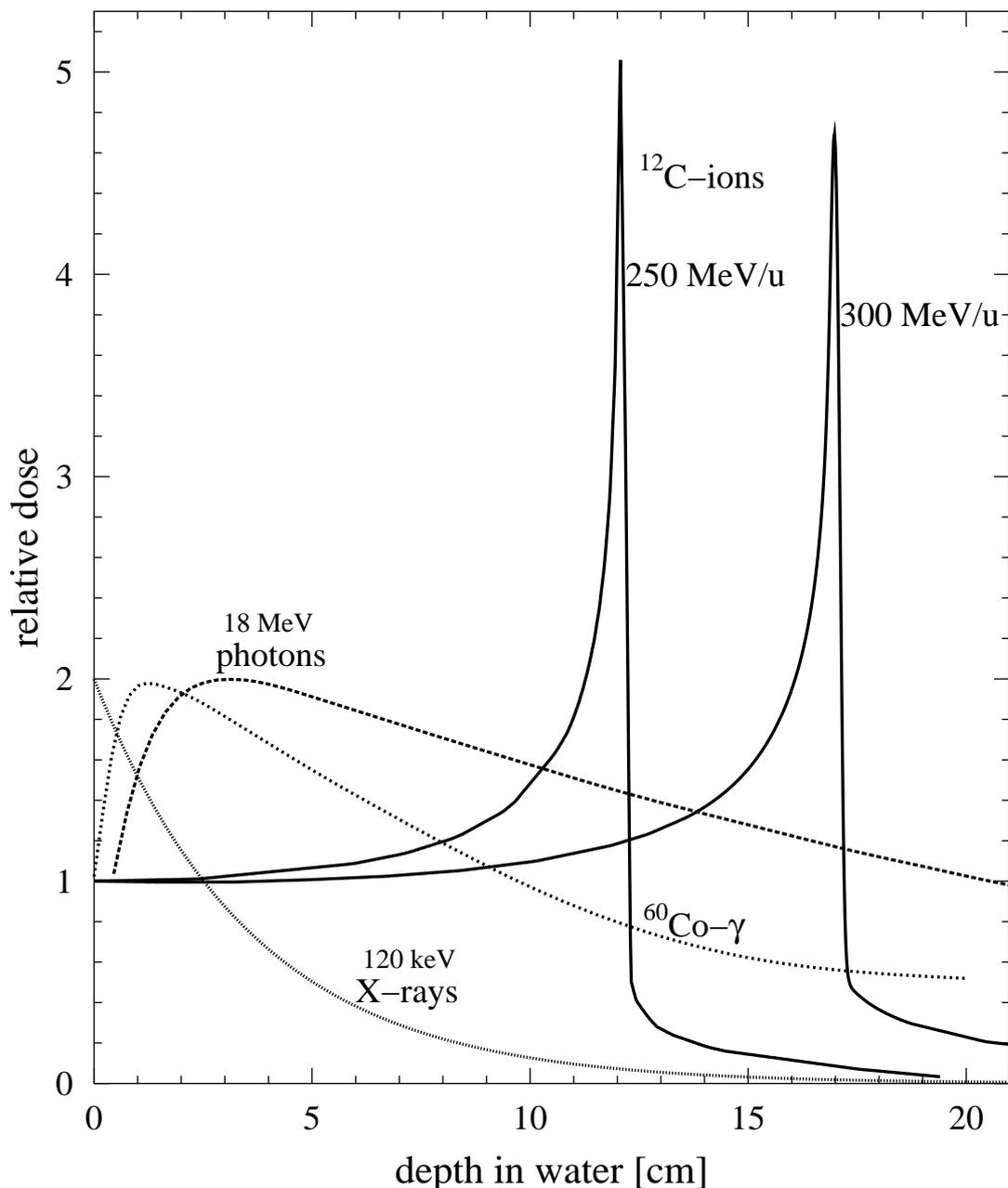
Fig. 1 Comparison of the depth dose profiles of X-rays, Co-gamma and Röntgen-Bremsstrahlung with carbon ions of 250 MeV/u and 300 MeV/u [with the courtesy of U. Weber].
