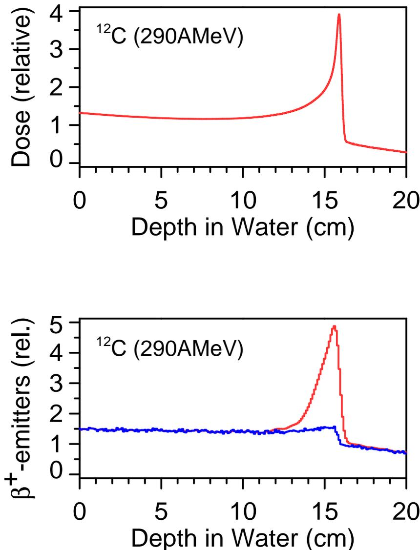
Fig. 8: The Bragg curve (top) is compared to a calculated  $\beta^+$  distribution expected for the irradiation of a PMMA absorber with a monoenergetic carbon ion beam. Bottom: the upper line displays the projectile fragments and the lower line the target fragments (with the courtesy of W. Enghardt).
