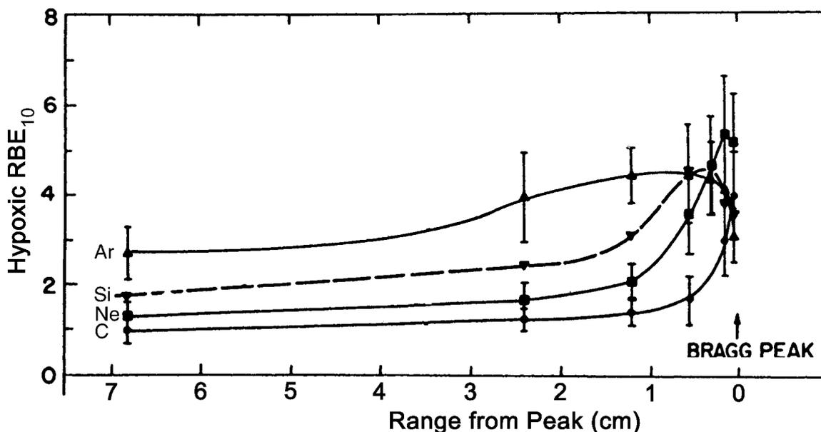
Fig. 2: RBE for C, Ne, Si and Ar ions as function of the penetration depth [redrawn from Blakely 1980]
